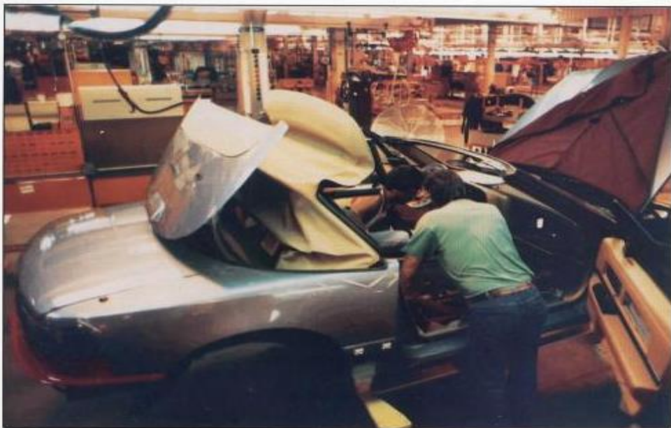
Reatta is hand built at the rate of about six cars per hour.
