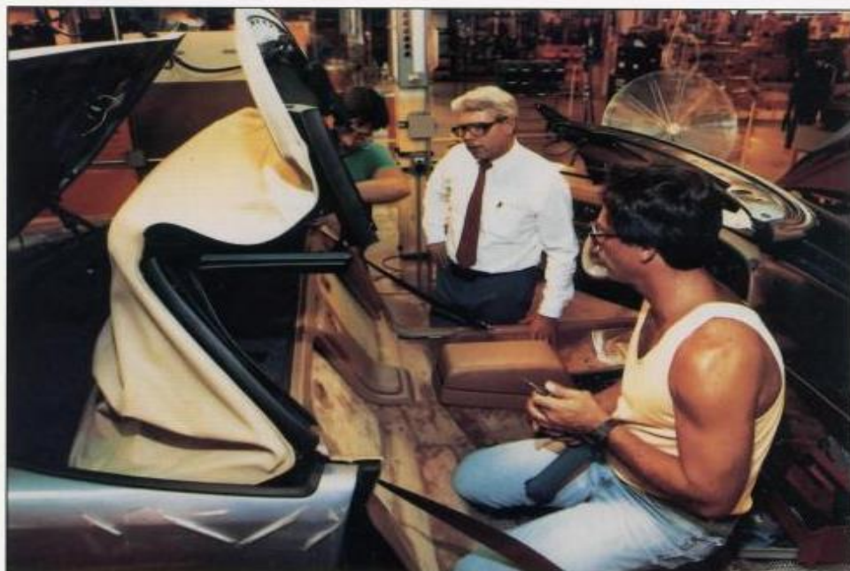
Plant manager Jim Rucker observes as Reatta craftsmen Robert Snow (left) and Ken Barber install a convertible top on a 1990 Reatta.
