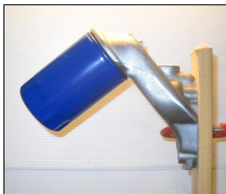
Blue filter shows the angle of the early 91 adaptor.
