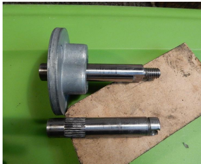
(1) with the green background shows the shaft and casting together with just a shaft below that shows the knurl.
